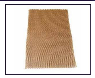
Aerospace grade Non-metallic honeycombs are made by forming aramid paper, which is high temperature resistant, into a honeycomb shape and coating it with phenolic resin.
