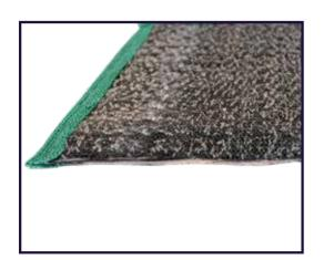
An intermediate layer of sodium bentonite powder is usually placed between two layers of non-woven geotextile that make up a geosynthetic clay liner (GCL), a mineral sealing mat that is manufactured by Hipex in ahedabad, Gujarat, India. A stitching procedure is used to link the two layers of geotextile (needle punched non-woven). With great internal shear resistance for a range of environmental confinement applications, this results in an utterly stable mat.
