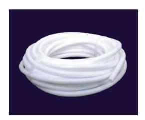
Our backer rod is made of extruded polyethylene foams, which are compressible, flexible, and durable enough to fulfill the stringent performance specifications of various applications. It is inserting to joint control sealant depth, creating a backstop to allow proper sealant tooling. It can also be used as a temporary joint seal. They are non-absorbent and can withstand most other sealants as well as oil and gasoline. The majority of cold-applied sealants are compatible with them.
