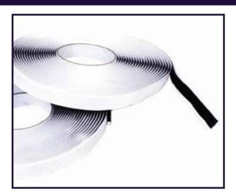
Low temperature sealant tape ideally utilized in vacuum bagging technique for making small component of composite product where temperature does not exceed up to 300°F (150°C). It has high cohesive Strength and sealing capability, as well as adhesion to a variety of films and tooling surfaces. It is compatible with a wide variety of film types and implements surfaces of aluminum, steel, fiberglass, nickel and graphite etc.
