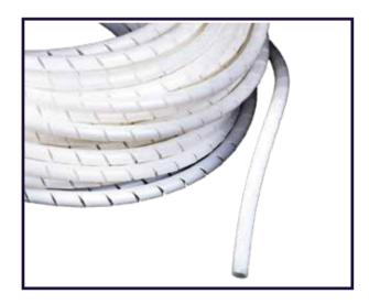
A spiral tube is an extruded plastic component that is frequently used to distribute resin evenly over a laminate or component during the infusion process. Resin may be supplied all the way along a composite edge because it flows readily through the middle of the spiral-finned tube and equally as easily out of the spirals on the side.
